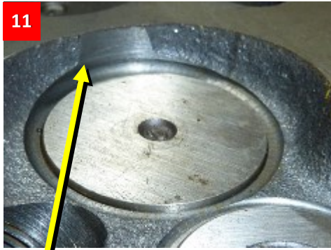
11. Witness mark made by the cutter does vary depending upon the cast chamber pocket position.
