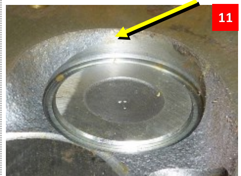
11. Witness mark made by the cutter does vary depending upon the cast chamber pocket position.
