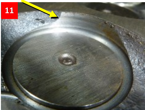
11. Witness mark made by the cutter does vary depending upon the cast chamber pocket position.
