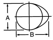
A: Inlet 27.66mm. Exhaust 27.93mm. B: 34.35mm.
