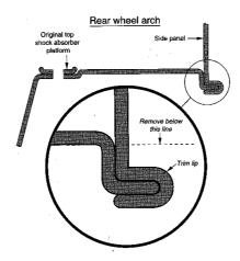
The original rear shock absorber platform must always remain in its original position. See also TR 5.6.1.17.
